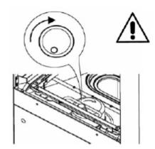
WARNING: In case of wrong direction of rotation, the mechanical to ensure the shift is ineffective.
